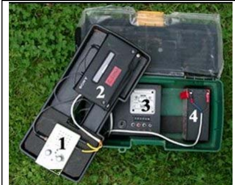
(1) D140 bat detector (2) tape recorder (3) "black box" (4) battery
